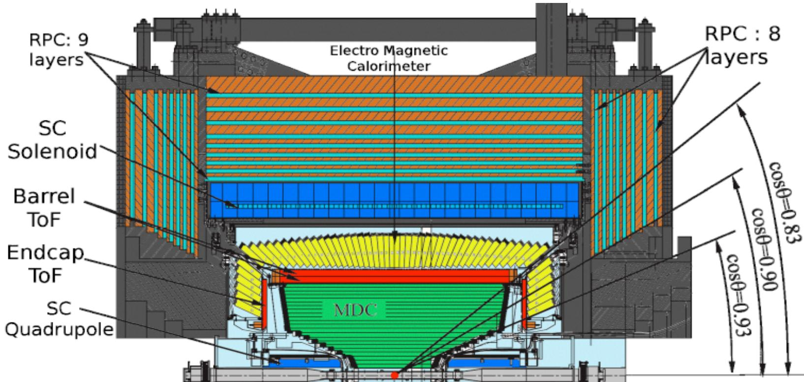
Wire tracker (no Si); TOF +  $dE/dx$  for PID; **CsI Ecal**; RPC muon
