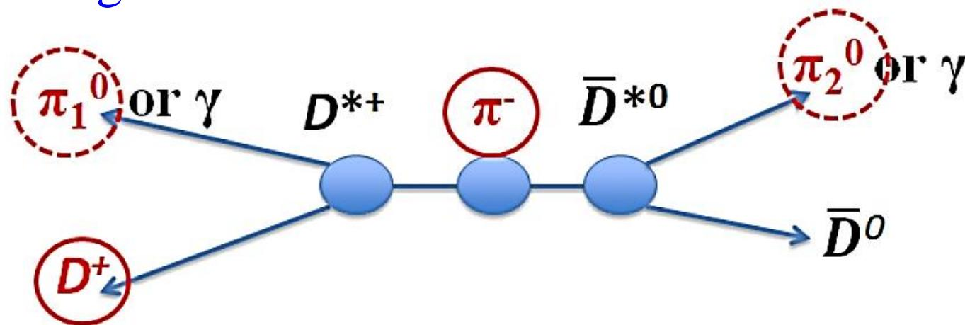
Topology of the decays of the signal process. Thick line circled  $D^+$  and  $\pi^-$  are detected in the final states and at least one of the dashed line circled  $\pi_1^0$  or  $\pi_2^0$  is tagged.
