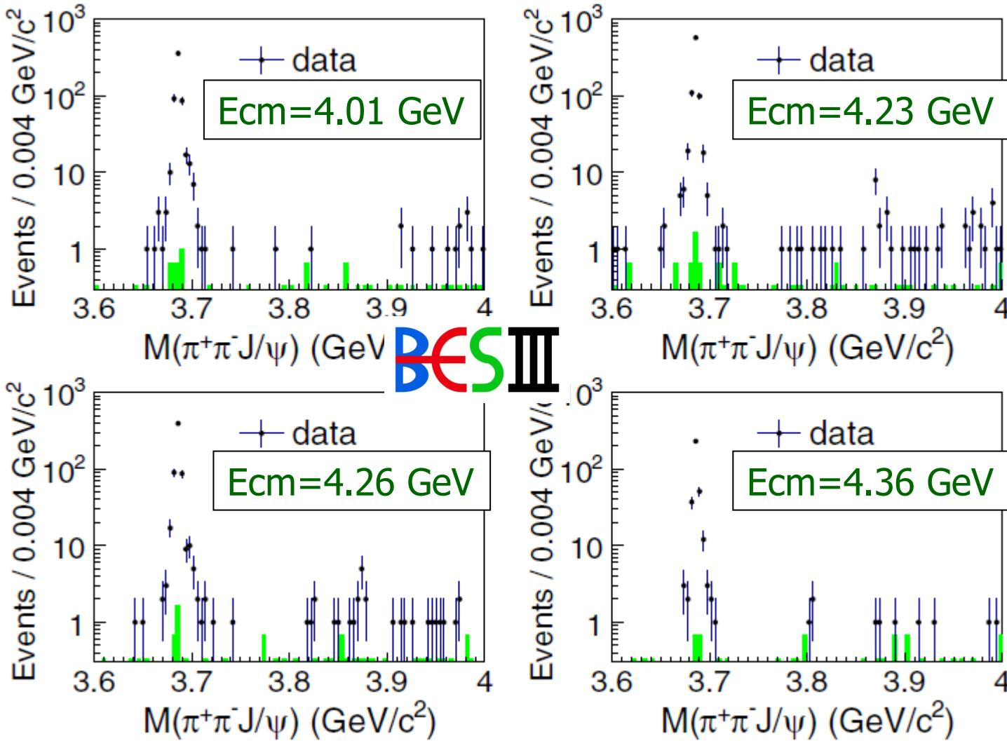
Clear ISR  $\psi'$  signal for data validation X(3872) signal at around 4.23-4.26 GeV
