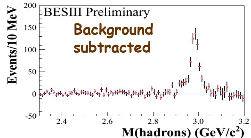
The  $\eta_c$  lineshape is not distorted in the  $h_c \rightarrow \gamma \eta_c$ , non-resonant bkg is small. This channel will be best suited to determine the  $\eta_c$  resonance parameters.
